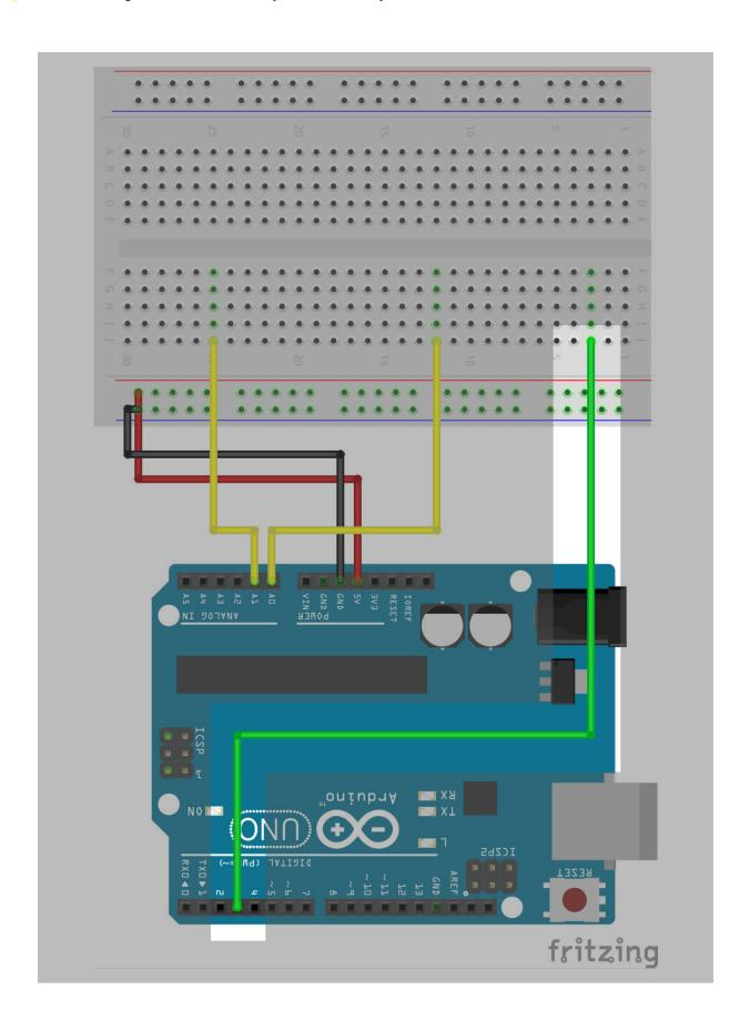
4 Place the potentiometer on the breadboard, so that the middle leg is on the same vertical line as the yellow wire connected to A0. Connect a red wire from the first potentiometer leg to the second row of your breadboard, and a black wire from the third potentiometer leg to the first row of the breadboard.
