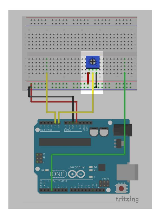
5 Place the resistor so that its right leg is on the same vertical line as the yellow wire connected to A1. Connect a red wire from the first left resistor leg to the second row of your breadboard, and a black wire from the middle of resistor to the first row of the breadboard.
