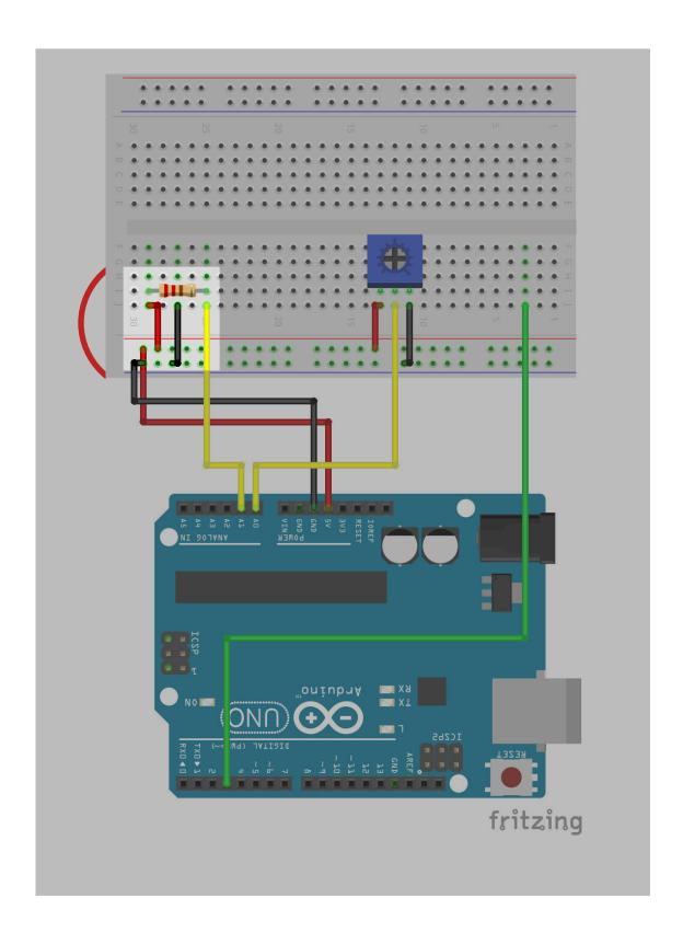
Place one red jump wire, one black jump wire and one yellow jump wire before the resistor, on the same vertical line as the wires you just added. Connect them to your hall effect sensor using matching colored alligator clip wires. Make sure the curved side of the sensor is facing you.
