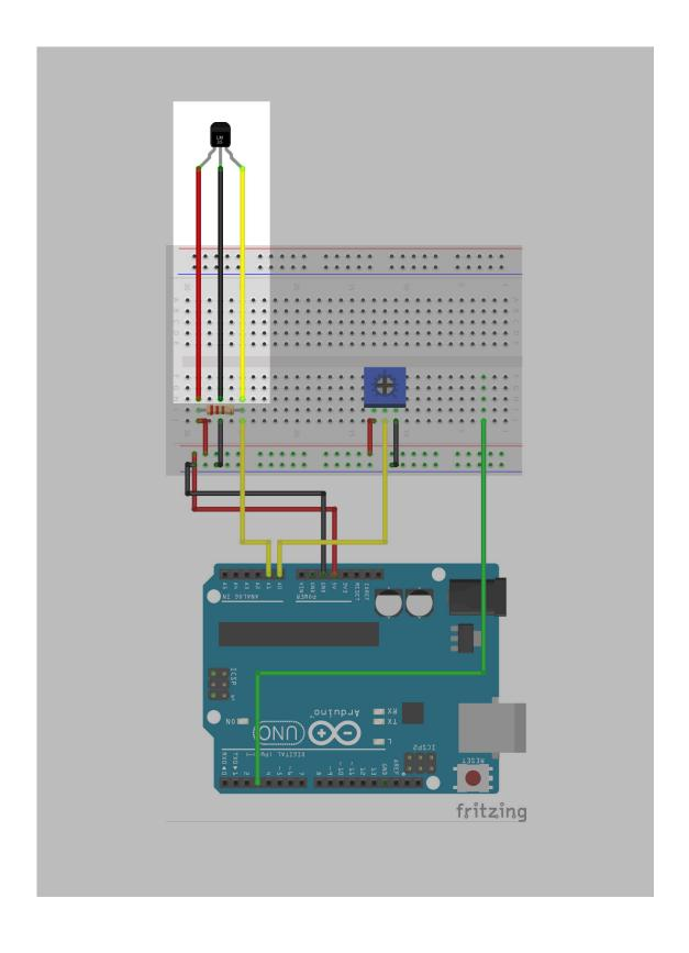
7 Place another green wire on the same vertical line as the green wire connected to ~3 and a black wire on the first row of the breadboard. Connect one side of the electromagnet to the green wire using a matching green alligator clip and the other end to the black wire using a matching black alligator clip.
